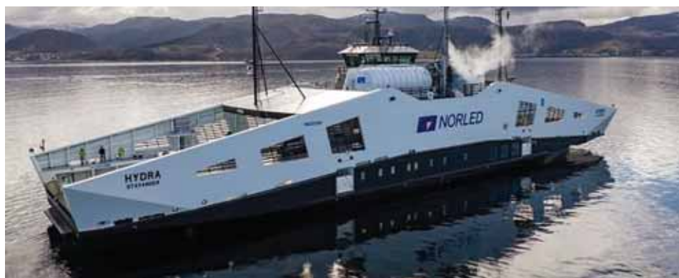
The MF Hydra , powered by fuel cells, has successfully completed sea trials and is now in commercial operation. Credit: Norled
