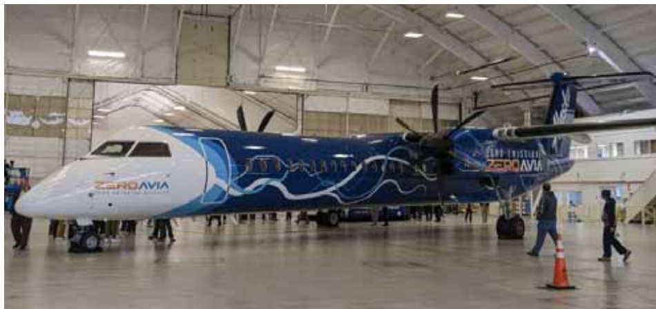
Alaska Airlines has provided ZeroAvia with a Dash 8 Q400 regional turboprop to test its hydrogen-powered electric propulsion system. The plane is now emblazoned with ZeroAvia navy- and sky-blue graphics and Alaska Airlines' name on the tail. Credit: GeekWire Photo / Lisa Stiffler
