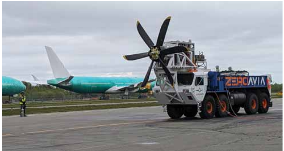
ZeroAvia's ground-test truck outfitted with two of its 900-kW (kilowatt) engines and a Q400 propeller. Credit: GeekWire Photo / Lisa Stiffler
