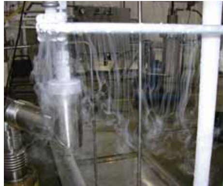
Liquid hydrogen transfer operation showing transition from vacuum jacketed line to uninsulated vent line. Credit: J. Fesmire
