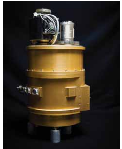
Mineral and gas identifier (MAGI) is a wide-swath moderate spectral resolution thermal-infrared imaging spectrometer detector cooled to 55 K. Credit: Aerospace
